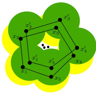
**Fig. 5** This figure illustrates a typical motion of the robots during herding phase. The robots moves from  $(x_1, x_2, x_3, x_4, x_5)$  to  $(x'_1, x'_2, x'_3, x'_4, x'_5)$ . Yellow circles depict the initial superlevel set, while the final one is depicted in green (Color figure online)
