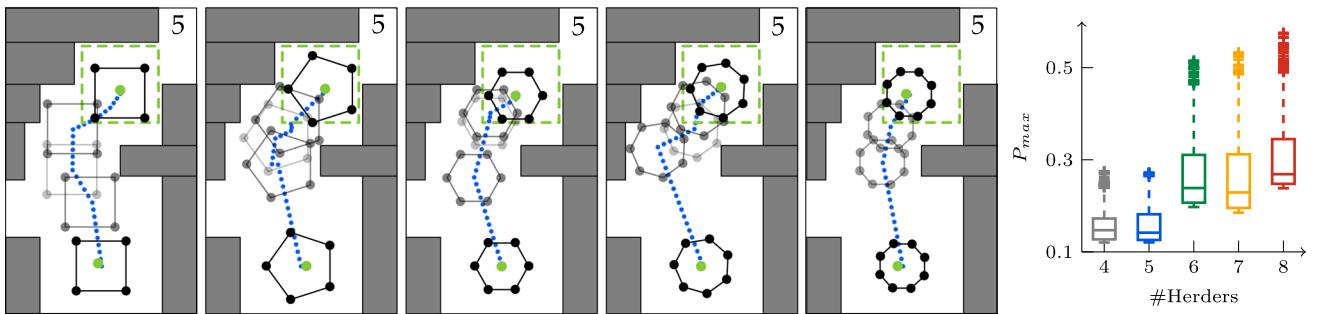
**Fig. 12** Herding experiments with different number of herders. Left: Herding path for 4–8 herders. Right: The maximum potential of the sheep has been sampled against all herders and were recorded during the whole process
