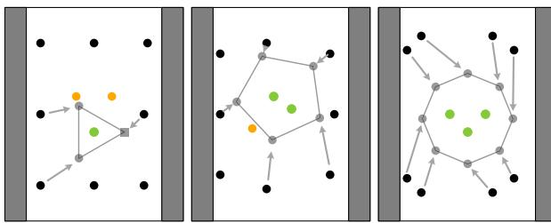
**Fig. 8** Initial cage acquisition path planning. Green dots mark the target sheep to be caged. Black dots are the initial positions of all the 8 standby herders, and gray dots are the positions of the selected herders when an initial cage is achieved (Color figure online)
