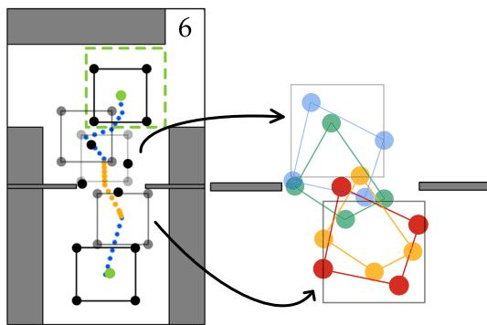
**Fig. 13** Herding experiment with team deformation. When passing through the narrow passage, the team deformation process is depicted by a close-up figure on the right. In the deformation procedure, the shape of the herding team was changing in the order of red, yellow, green and blue, and then resumed to the normal shape (Color figure online)
