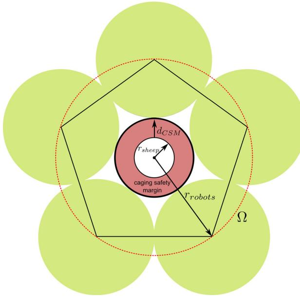
**Fig. 3** This figure depicts a caging chain formed by 5 robots.  $r_{sheep}$  is the radius of the circle which is guaranteed to contain the sheep at the current moment of time. Green circles represent the area of potential, greater or equal to the potential of the caging chain. The red region corresponds to the caging safety margin.  $r_{robots}$  is the radius of the caging circle  $\Omega$  (Color figure online)
