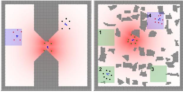
**Fig. 16** The obstacles are depicted in grey; the goal region is the blue square; the black dots correspond to the initial configuration of the robots, the green dots depict the current configuration, and the red dots are the robots in the final configuration. The potential field induced by the current configuration is depicted in red. In the second environment, the 3 remaining goals are depicted in green (Color figure online)
