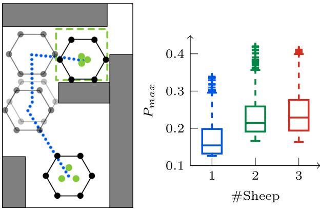
**Fig. 11** Herding experiments with different number of sheep. Left: The herding path generated by the algorithm for 6 herders. Right: The maximum potential of the sheep has been sampled against all herders and were recorded during the whole process
