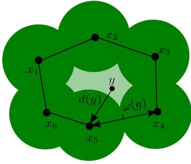
**Fig. 4** This figure depicts a caging chain formed by 6 robots.  $\omega(g)$  is the half of the length of the longest segment of the chain. Green circles depict the superlevel set of the potential function, containing the caging chain (Color figure online)
