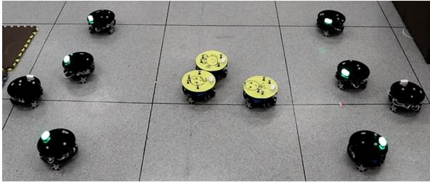
**Fig. 6** In our experiments, we use 8 mobile robots to act as herders (black) and 3 mobile robots to act as sheep (yellow). All the robots have the same radius of 0.12 m (Color figure online)
